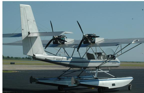
The aircraft is a twin engine kit plane which has an all up weight of under a ton. It is a parasol wing, wire braced design, with a tandem open cockpit. The minimally cowled Rotax engines are rated at 100 HP each and the aircraft is reputed to have rather phenomenal STOL capabilities. This particular model is equipped with amphibious floats. The manufacturer, Lockwood Aviation, is based in Florida and advertises a price of around 100 K. for the kit.
